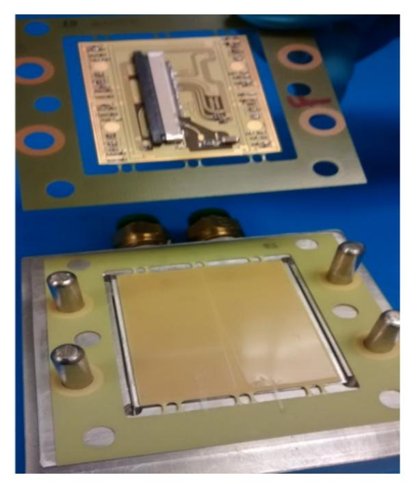
Using the flex cable jig, attach the detector module to the flex cable by exposing the other side of the epoxy.
