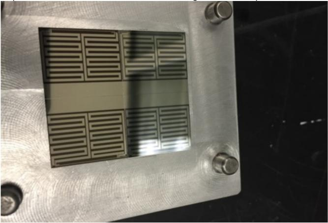
Now, place the other alignment plate on top. There should be a slight groove cut on one side of this plate, and this should face down.
