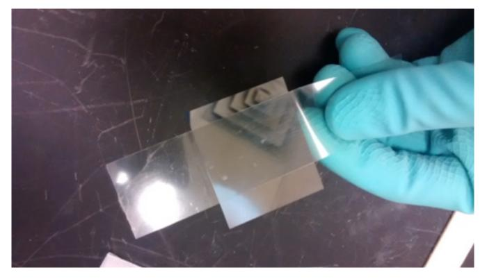
Now, remove the other side of the epoxy tape, and use the alignment jig to attach it to the front-end chips. In the case of a 1X2 module, you will only attach two of the front end chips and will want to align the silicon detector along the right hand side of the alignment jig to ensure enough space is left between the edge of the front end chips and the silicon detector.
