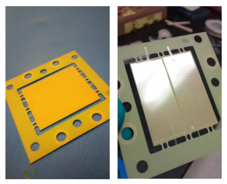
Now expose the epoxy tape after placing the secondary flex cable in the second jig. Then place the flex cable for use onto the exposed epoxy to transfer the tape correctly to the flex cable.
