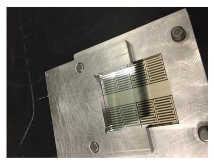
Remove one side of the double-sided epoxy and attach it to the silicon sensor. Then, use scissors to cut away the excess portion on either side.
