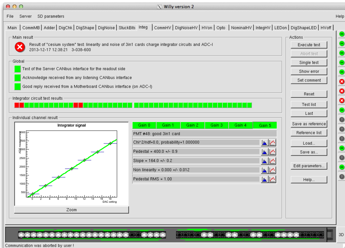
Figure 37: Example of the Integ read-out test with super-drawer in ATLAS
